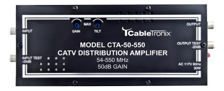
The CTA-50-550 is a professional quality broadband launch amplifier designed to produce clean signals for a commercial grade CATV network. Employing a push/pull design, the CTA-50-550 produces high output levels with extremely low distortion and harmonic content. As a broadband amplifier with a frequency range of (54-550)MHz, the CTA-50-550 supports CATV channels (2-78), with forward path amplification only.
